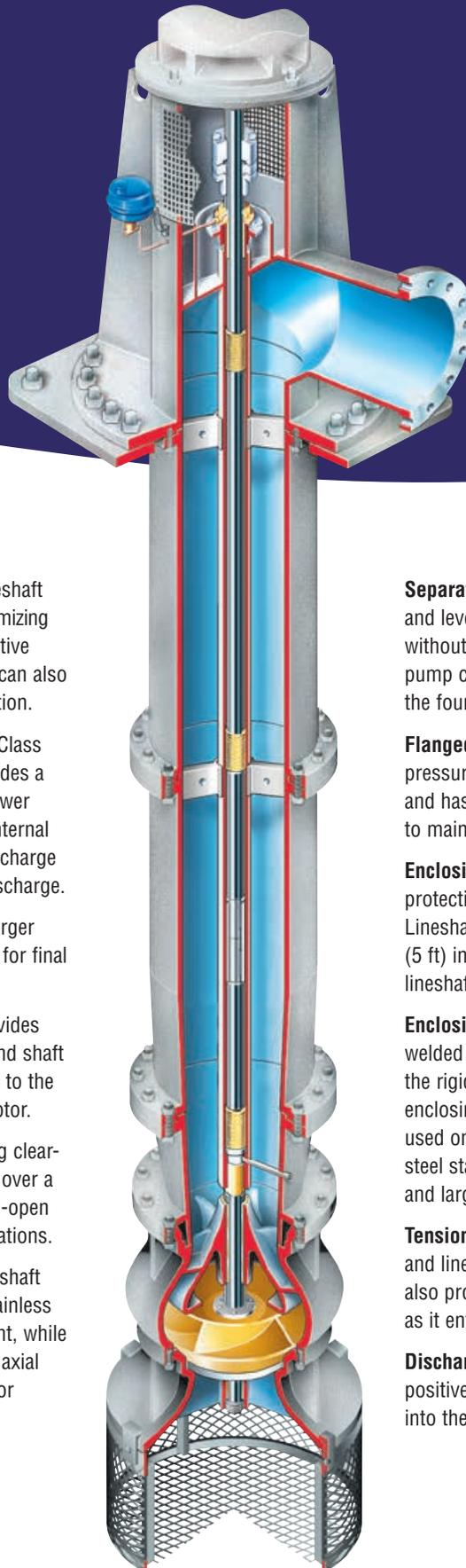
**Enclosed Oil Lubrication** isolates the lineshaft and bearings from the pumped liquid, minimizing maintenance in abrasive services. Alternative lubricants such as clean water or grease can also be used with enclosed lineshaft construction.
