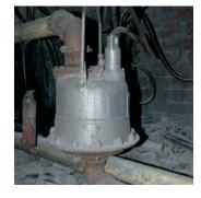
In-line staged submersible pump increases pumping distance.
