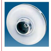
High Efficiency Semi-Open or Closed Impellers in standard glass reinforced polymer or optional cast iron, bronze or 316 SS to suit service conditions. Impellers are keyed to shaft for positive drive and provide maximum efficiency
